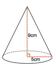
Volume of cone  $=\frac{1}{3}\pi r^2 h$ Curved surface area of cone  $=\pi rl$
